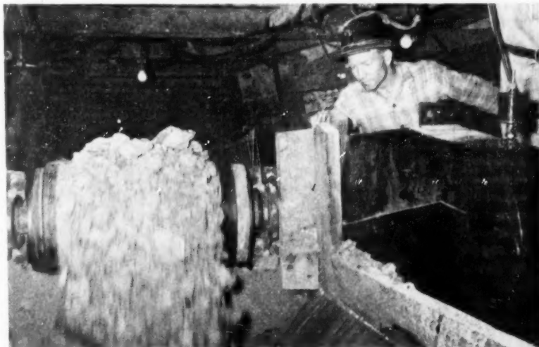
J. D. Manues watches the level of ore in the hopper feeding to the main haulage level. When the bin is full the conveyor is stopped; scrapers on the level above are coordinated with the conveyor by an automatic system of signal lights.
